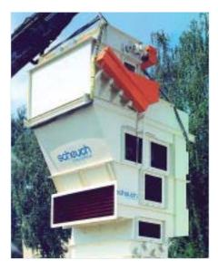
Scheuch first turned its attention to the topic of airstream sorting some 10 years ago and developed the SWSF fibre classifier (SWSF = Scheuch-Wind-Sichter für Fasern) for use in the production of MDF board. Its job is to clastions and ensures the high quality of the MDF sheets, which is especially important in the case of thin sheets.
